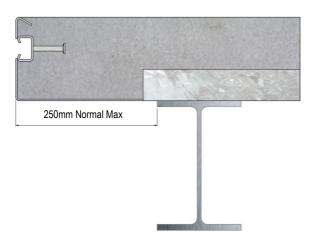
For larger cantilevers it may be necessary to provide temporary propping until such a time as the slab has achieved its required strength.
