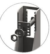
offset hole in the washer allows the increments of adjustment to be halved when rotated through 180° meaning the support level can be finely adjusted by +/- 30mm. The design of the Alpha System provides clear inspection into the location and engagement of the washer in the bracket simplifying the final site installation checks.
