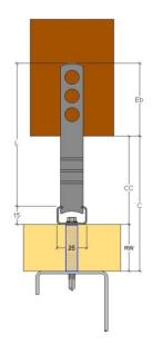
An ACS 4000 Range Channel Tie should be selected to ensure a minimum of 50mm and a maximum of 75mm is selected to ensure that the minimum embedment of 50mm is always achieved. ACS recommends that ties should be selected to an embedment (Eb) of 62.5mm.
