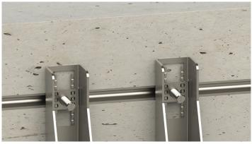
6. Each bolt should be turned 90° to lock in place. The notch in the bolt shank should be vertical.
