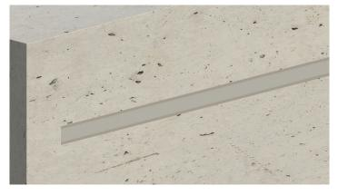
1. After the concrete is poured, it should be left to cure with the insert left in place.
