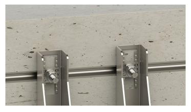
Nuts and form B washers can then be loosely placed onto the 7. bolts and the level adjusted as required. The alpha washer can be spun 180° to allow for fine adjustment if required. The nut can then be tightened to the correct torque setting of 25Nm.
