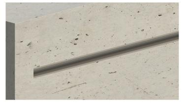
No filler or concrete should be left within the channel. Any 3. remaining concrete should be scraped out. It is important that no power tools are used for this and sufficient care is taken of the concrete in the surrounding area.
