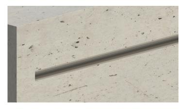
No filler or concrete should be left within the channel. Any remaining concrete should be scraped out. It is important that no power tools are used for this and sufficient care is taken of the concrete in the surrounding area.
