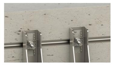
Nuts and form B washers can then be loosely placed onto the bolts and the level adjusted as required. The alpha washer can be spun 180° to allow for fine adjustment if required. The nut can then be tightened to the correct torque setting of 25Nm.
