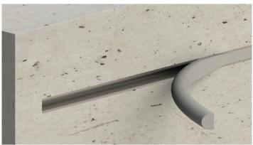
After the formwork has been struck, the filler should be removed from the channel.
