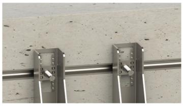
Each bolt should be turned 90° to lock in place. The notch in the bolt shank should be vertical.
