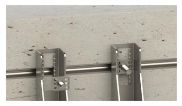
31/21 T Head Bolts should be inserted through an alpha washer and into the channel through the slot in the back of the bracket.
