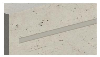
After the concrete is poured, it should be left to cure with the insert left in place.
