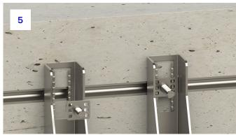
**5.** 31/21T Head Bolts should be inserted through an alpha washer and into the channel through the slot in the back of the bracket.
