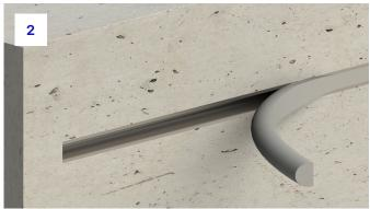
**2.** After the formwork has been struck, the filler should be removed from the channel.
