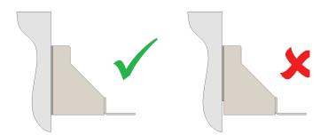
The maximum allowable thickness of the shims should not exceed the outside diameter of the fixing. As ACS Masonry Support systems typically utilise 12mm diameter fixings, this tends to be the maximum allowance. If more than 1No. shim is required, it is important that the total number of shims is kept to a minimum to avoid creating slip planes that may allow settlement or creep under load.
