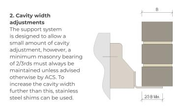
When utilising these, it is important that the shim is fully bearing on the structure to support the compressive forces at the heel of the bracket.
