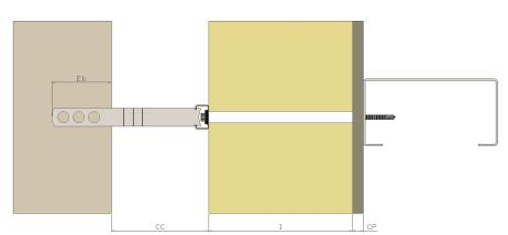
Although ACS Framefix™ channel is supplied in 2.7m lengths, it is likely that smaller pieces will be required on site. The channel can be cut down on site as required, however there must always be 2no. fixings minimum in the length of channel.
