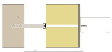
Although ACS Framefix $^{\text{\tiny{M}}}$  channel is supplied in 2.7m lengths, it is likely that smaller pieces will be required on site. The channel can be cut down on site as required, however there must always be 2no. fixings minimum in the length of channel.
