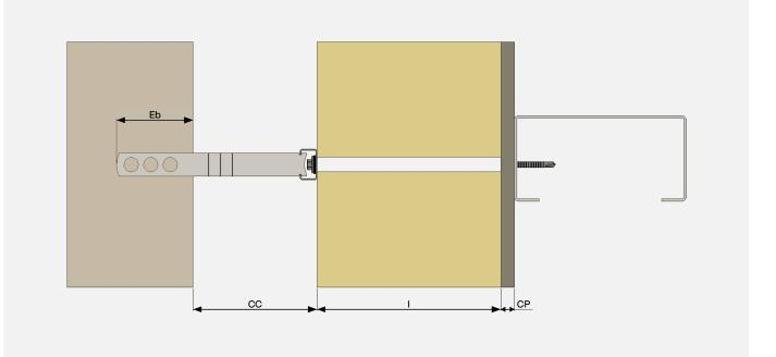
Although ACS Framefix<sup>™</sup> channel is supplied in 2.7m lengths, it is likely that smaller pieces will be required on site. The channel can be cut down on site as required, however there must always be 2no. fixings minimum in the length of channel.
