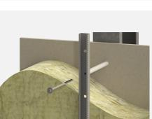
**3.** Install fixing through channel and sleeve back to internal structure.
