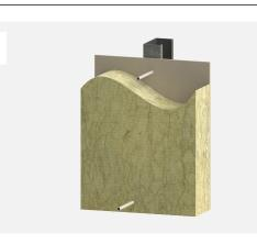
**1.** Mark out and install sleeves through insulation at centres shown in table 1.0.
