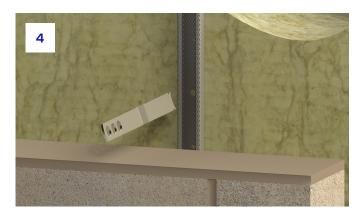
4. Rotate ACS 4000 range tie into channel lips.
