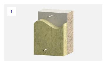
**1.** Mark out and install sleeves through insulation at centres shown in table 1.2
