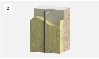
**2.** Drill pilot hole at diameter shown in table 1.2 at each fixing location
