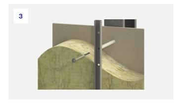
**3.** Install fixing through channel and sleeve back to internal structure.
