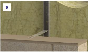
**5.** Embed tie into the mortar joint.
