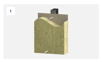
**1.** Mark out and install sleeves through insulation at centres shown in table 1.0.
