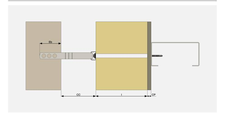
Although ACS Framefix™ channel is supplied in 2.7m lengths, it is likely that smaller pieces will be required on site. The channel can be cut down on site as required, however there must always be 2no. fixings minimum in the length of channel.
