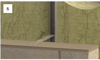
**5.** Embed tie into the mortar joint.
