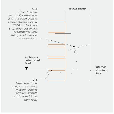
GT2 - This is a single sloping planar metal sheet which acts to dissipate moisture away from the inner leaf of the cavity wall. Its shape ensures water flows from the cavity towards the horizontal GT1 component embedded in the outer leaf of masonry. To aid the stability of the G-Tray<sup>™</sup>, the upstand section is fixed to the internal leaf.
