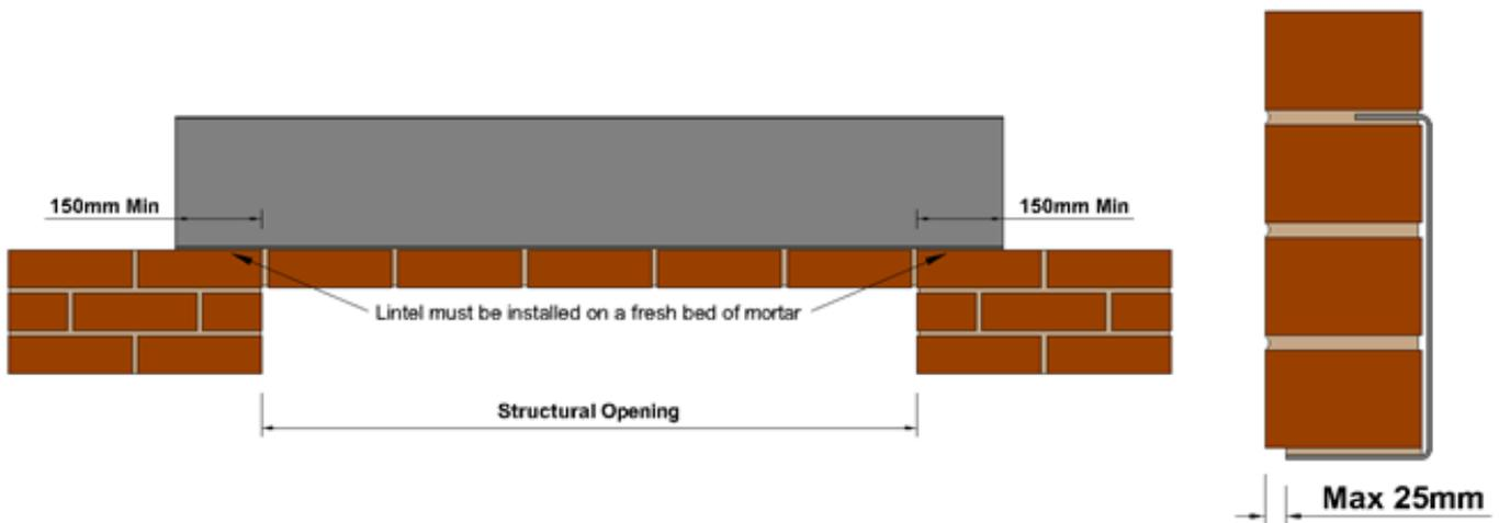
Lintels should always be propped during construction to achieve the safe working load capacities declared in the design tables below. A separate DPC is required above the lintel.
