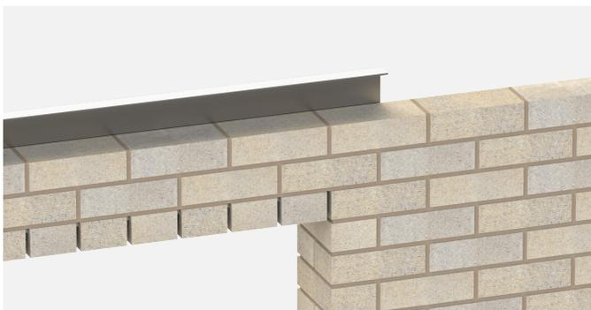
Lintels should always be propped during construction to achieve the safe working load capacities declared in the design tables found within this document.
