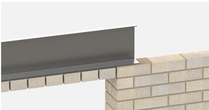
A minimum of 150mm end bearing must be achieved at either end of the lintel unless specified otherwise by ACS. A maximum masonry overhang of 25mm over the front edge of the lintel must also be maintained.
