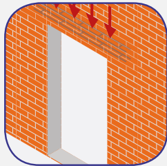
Masonry lintels doors
