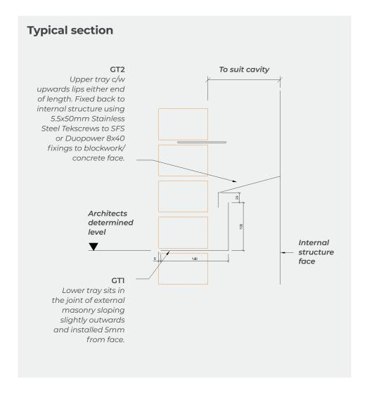
GT2 - This is a single sloping planar metal sheet which acts to dissipate moisture away from the inner leaf of the cavity wall. Its shape ensures water flows from the cavity towards the horizontal GT1 component embedded in the outer leaf of masonry. To aid the stability of the A-Tray™, the upstand section is fixed to the internal leaf.
