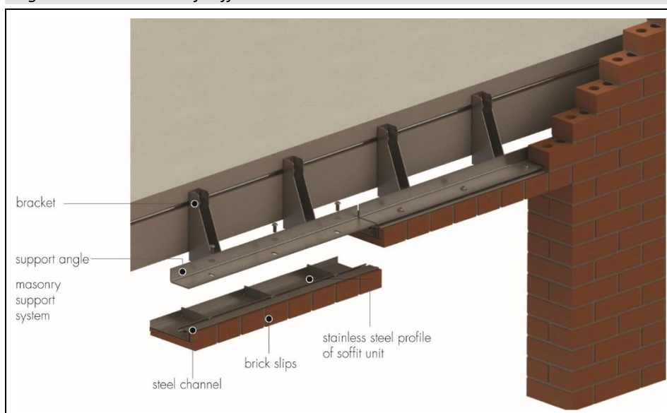
Figure 11 Installation of soffits
