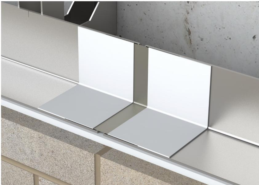
Between each masonry support angle is located a circa 10mm gap to allow for building tolerances. To counter this from a moisture perspective, a separate Intex™ jointing piece is used to bridge the gap. This is attached in the same manner as the ACS cavity tray products, with both a double-sided butyl tape between the angle and jointing piece, as well as a single-sided butyl tape over the top of the joint. This has been independently assessed as part of the Kiwa third-party certification.
