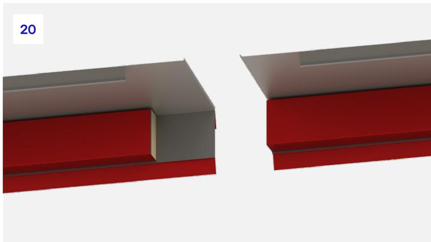
**20.** You will now have a rear barrier with a full end attached to the brackets and an additional cut piece ready for installation.
