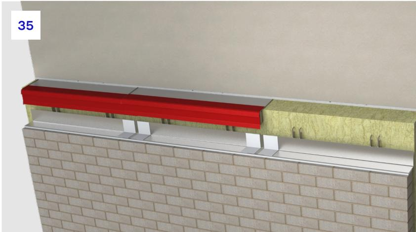
**35.** Once in place, to ensure rear components are touching, the second barrier must be slid toward the first barrier, utilising the system tolerance.
