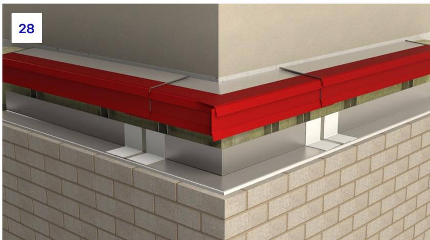
**28.** Once the second tray is in place, the same process can be followed for any remaining trays, ensuring the references match between the drawing, angle, and tray.
