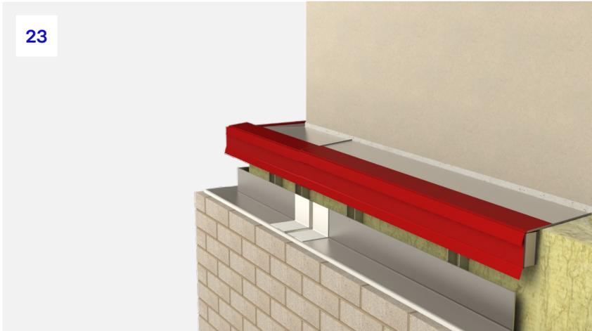
**23.** Once in place, to ensure rear components are touching, the second barrier must be slid toward the first barrier, utilising the system tolerance.
