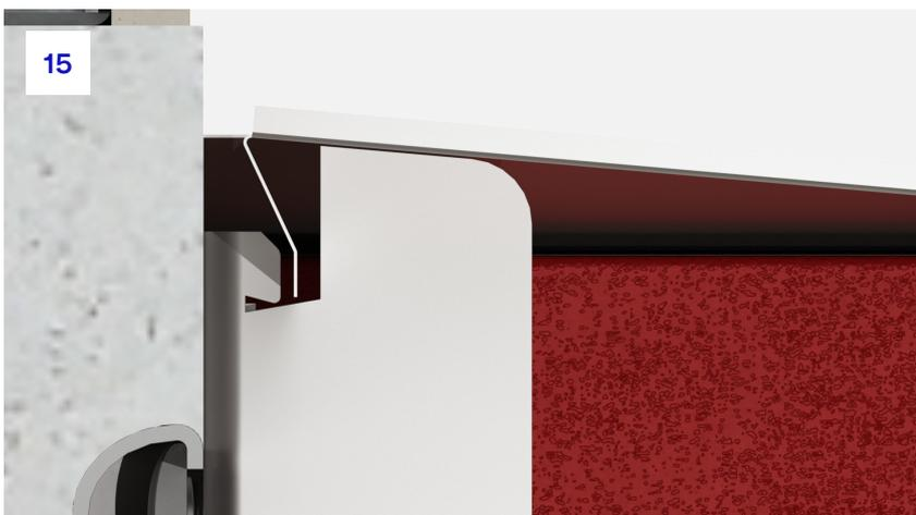
**15.** On the left-hand side of the corner tray, the formed section is just required to sit within the gap of the bracket notch allowing the tray to be restrained in place laterally.
