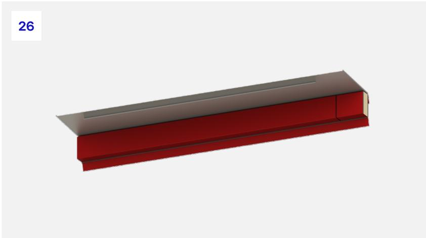
**26.** The mark should be continued around the rear section of the barrier so it is clear where the barrier needs to be cut.
