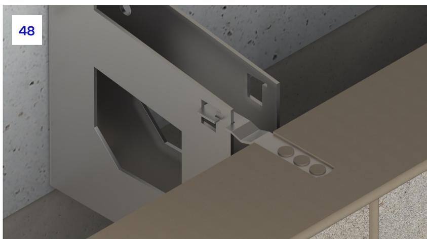
**48.** The Intex™ tie should be pushed downwards and embedded into the mortar ensuring it is pushed into the centre of the joint.
