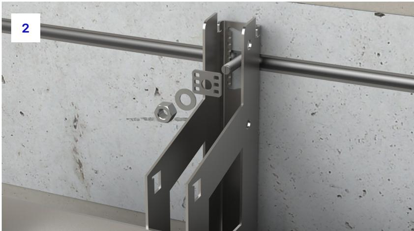
**2.** A fixing should be inserted through the bracket into the structure. For reference, ACS 31-21 cast in channel has been shown; however, please follow fixing specific installation instructions. Upon this fixing should be located an alpha adjustment washer which will allow for vertical tolerance, as well as a form B washer and hex head nut.
