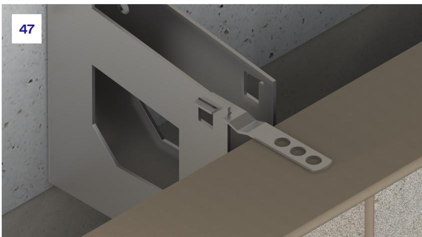
**47.** The Intex™ tie should then be lowered down the bracket notch into the lower section. Tolerance is within the notch to allow for both standard bricks as well as pistol bricks.
