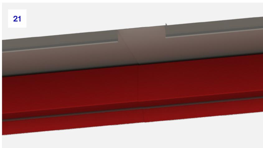
**21.** Once the rear barrier is cut the two barriers can be pushed together. For the rear section, the two barriers should be fully butted together to ensure they provide a continuous stop against heat and flame. It is imperative that the barriers are fully butted together at this stage.
