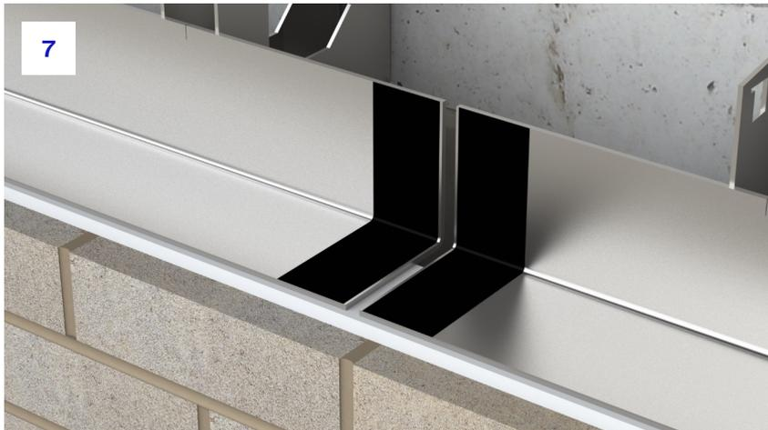
**7.** Utilise a strip of double-sided ACS Butyl tape on the end of each angle. This tape should be located at the end of the angle and should cover the full height and depth of the section to ensure full coverage against water. The tape has a top covering release layer that should be kept in place at this stage. Ensure that the tape is fully adhered to the angle. Once in place, the release tape can be removed.
