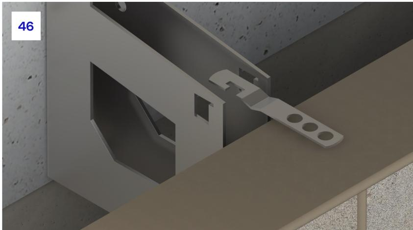
**46.** To ensure restraint of the masonry panel, the brackets include specially designed notches to allow Intex™ ties to be installed. The tie should be clipped into the bracket with the tie drip pointing downwards. This ensures that any moisture that may land on the tie is not carried towards the internal face of the cavity. The bracket notch is larger at the top and allows the tie to easily be clipped in.
