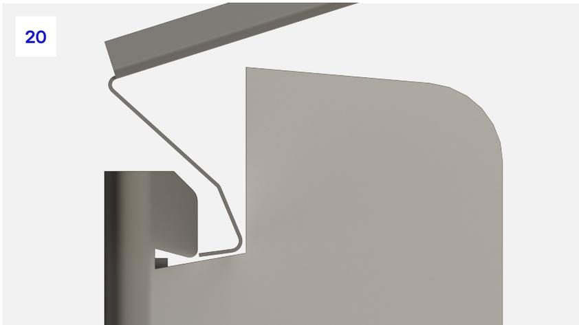
**20.** The bottom lip of the tray section should be pushed fully into the bracket notch to its rearmost face. The bracket notches are specially designed to match the profile of the tray.
