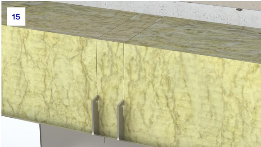
**15.** To the next side of the bracket, a piece of insulation should be installed again up to the bracket to ensure continuity.
