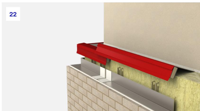
**22.** In the same manner as the first tray, the formed section of the tray can be placed into the bracket notches and rotated into place. The bottom lip of the tray section should be pushed fully into the bracket notch to its rearmost lip. The bracket notches are specially designed to match the profile of the tray. The tray can be fitted around the insulation ensuring a tight fit between all components.
