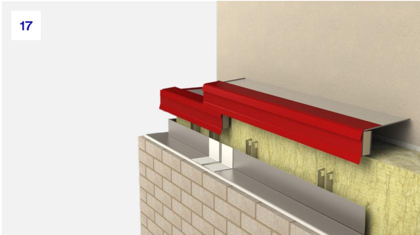
**17.** The next tray can then be placed on top with a minimum of 80mm overlap between components. Horizontal tolerance in the system is given by sliding the tray along the bracket slot on top in the required position, ensuring a minimum overlap of 80mm, mark the rear barrier where the two barriers meet.
