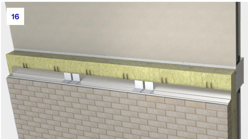
**16.** When complete, there should be a solid face of insulation across the façade, creating a continuous face for the rear intumescent to expand against.
