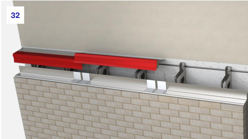
**32.** In the same manner as the first tray, the formed section of the tray can be placed into the bracket notches and rotated into place. See pages 13 and 14 for more details.
