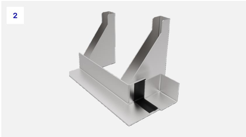
2. Over the top of the angle end utilise an Intex<sup>™</sup> stop end which will sit tight behind the return brickwork. This should overlap the angle by a minimum of 50mm. The piece allows for adjustment for required site tolerance.
