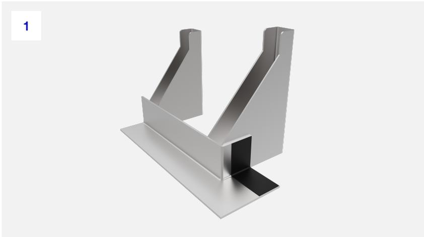
1. Utilise a strip of double-sided ACS Butyl tape on the end of the angle. This tape should be located at the end of the angle and should cover the full height and depth of the section to ensure full coverage against water. The tape has a top covering release layer that should be kept in place at this stage. Ensure that the tape is fully adhered to the angle. Once in place, the release tape can be removed.
