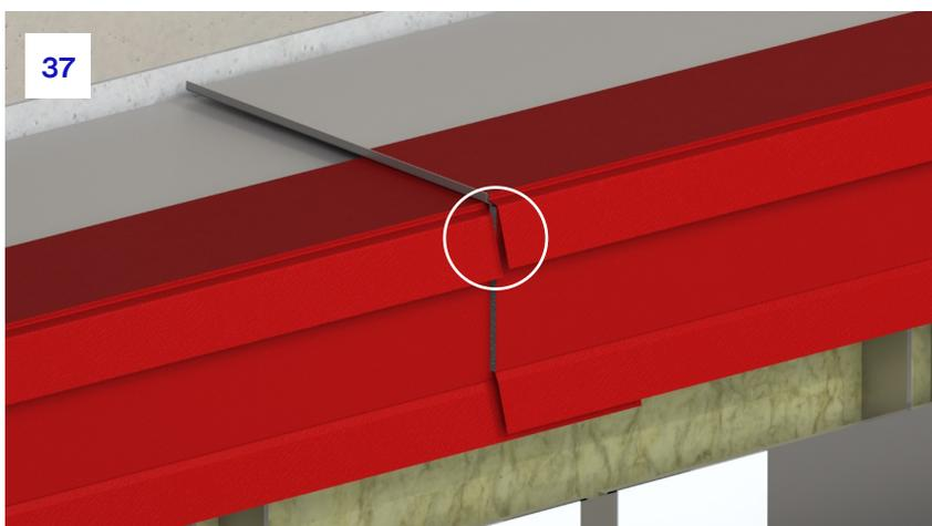
**37.** Once in place, the top wing should be cut tight to the tray lip to ensure it can move freely in the case of fire.
