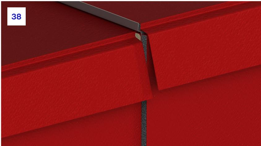
**38.** Once cut, the wing will be free to expand in the case of fire.
