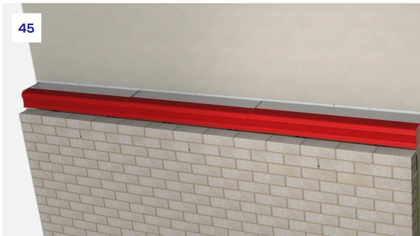
**45.** Brickwork may continue up the façade following industry guidance around maximum builds per day.
