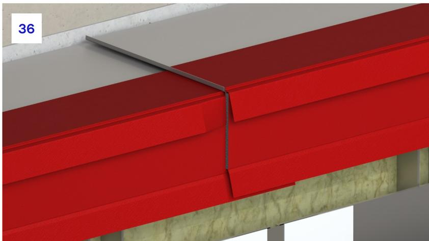
**36.** For both the top and front sections of the tray barrier, the second tray should sit on top of the lower barriers as shown in the image. This ensures continuity in the case of fire.
