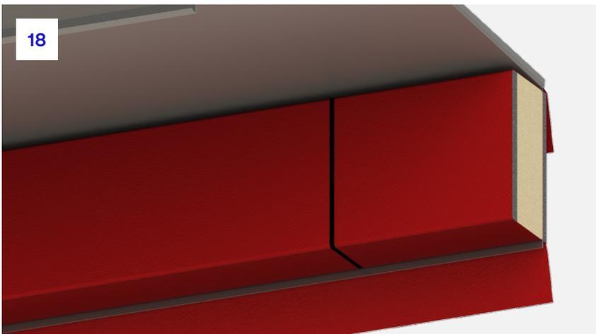
**18.** The mark should be continued around the rear section of the barrier so it is clear where the barrier needs to be cut. By creating a clear mark, this ensures cutting is easy to achieve and reduces the risk of errors.
