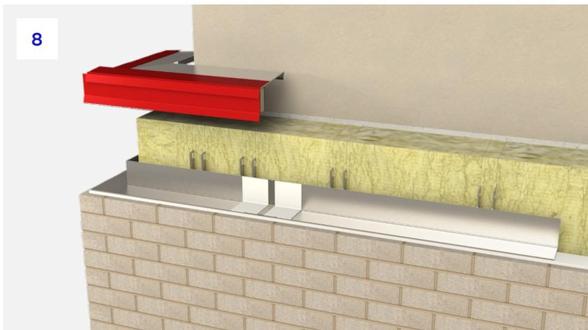
**8.** Once the insulation is in place, it is time to start the installation of the trays. The corner piece should be installed first and lined up with the brackets located below.
