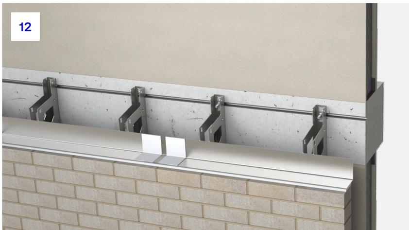
**12.** Once complete and the tape is sufficiently adhered, this gives a full barrier against moisture ingress.
