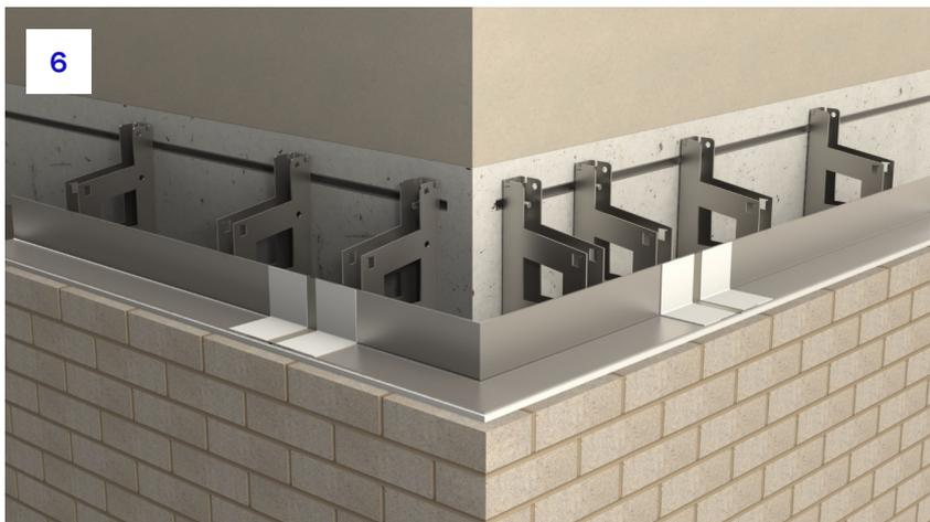
6. Install Intex™ jointing pieces over all gaps between angles. This requires a double-sided ACS Butyl tape each side of the gap, an Intex™ jointing piece, and a single-sided ACS Butyl tape for each side of the jointing piece. For further details, please see the main section of the installation guide.
