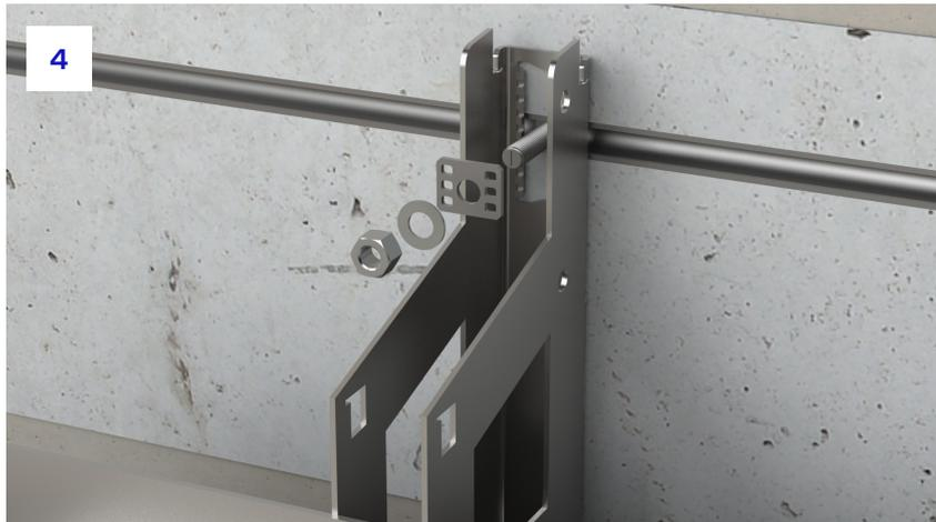
**4.** A fixing should be inserted through the bracket into the structure. For reference, ACS 31-21 cast in channel has been shown; however, please follow fixing specific installation instructions. Upon this fixing should be located an alpha adjustment washer which will allow for vertical tolerance, as well as a form B washer and hex head nut.
