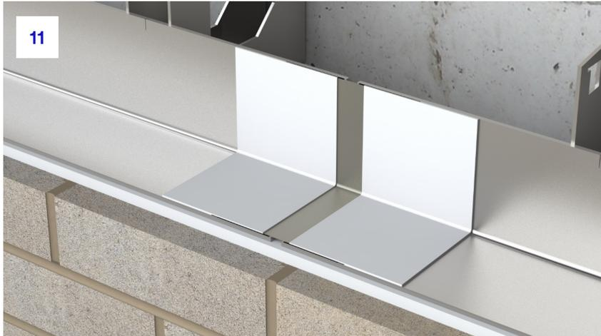
**11.** The tape should be pushed into the joint to ensure good adhesion and to stop the passage of any moisture.
