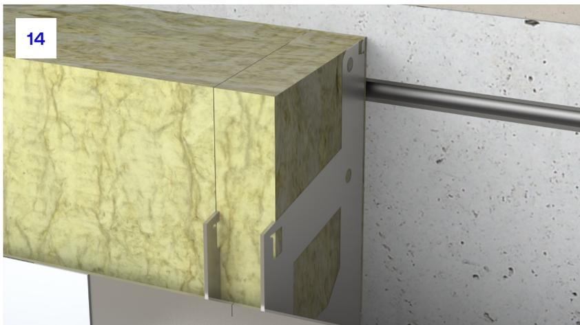
**14.** A further piece of insulation should be installed within the bracket ensuring it fully meets the adjacent insulation.
