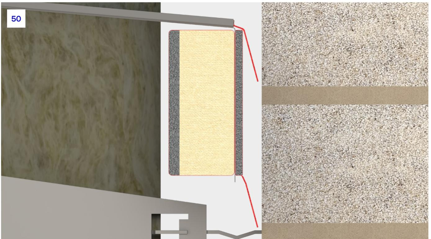
**50.** As brickwork continues up the façade, it is imperative that the barrier wings are left free within the cavity space. Under heat and fire, the wing expands into the brickwork to assist with intumescent expansion.
