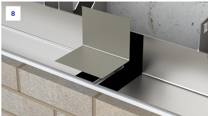
**8.** Over the top of the joint utilise an Intex™ jointing piece to bridge the gap. This should overlap each angle by a minimum of 50mm. The piece allows for adjustment either way to allow for site tolerance.
