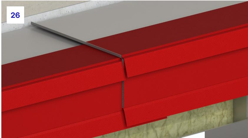
**26.** Once in place, the top wing should be cut tight to the tray lip to ensure it can move freely in the case of fire.
