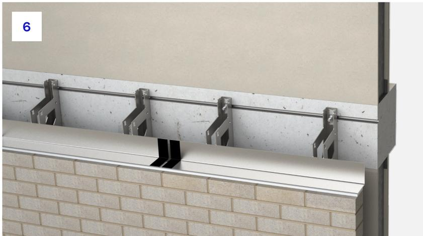
6. Once the Intex™ brackets and angles have been installed, it is necessary to create a continual barrier against moisture ingress. This is completed by using Intex™ jointing pieces and relevant sealing tapes.
