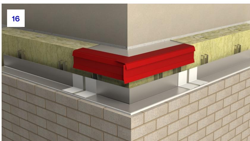
**16.** Once in place, the tray will be tight against the insulation and sat within all bracket notches.
