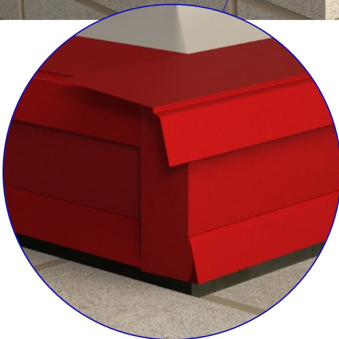
**31.** Brickwork should be built up to the level of the barrier and the wing on the front intumescent strip pushed inboard of the brickwork line. The wings should under no circumstance be built into the brickwork itself. More detail can be seen in the image below.
