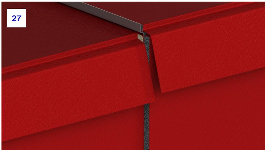
**27.** Once cut, the wing will be free to expand in the case of fire.
