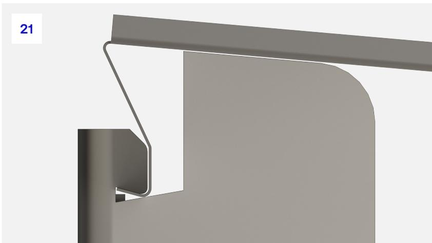
**21.** Once inserted into the slot, the tray can be rotated around to meet the top of the bracket notch and hold it securely in place.
