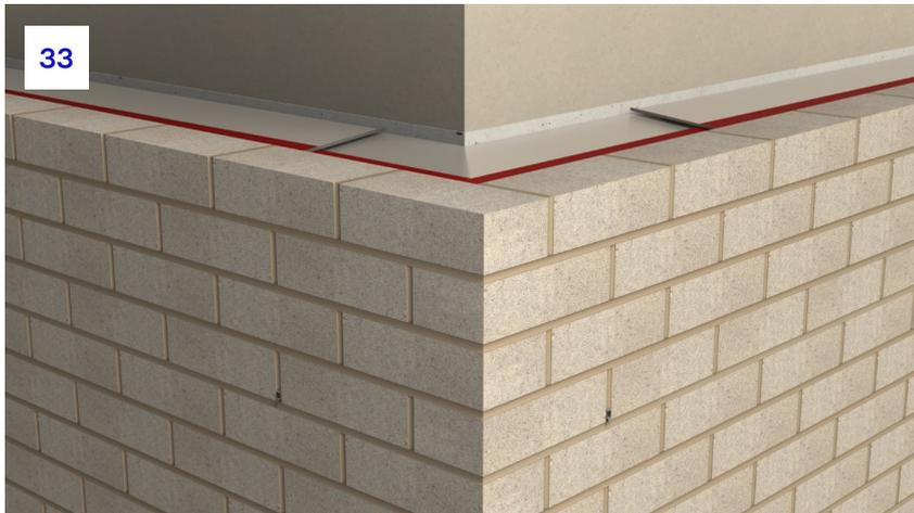
**33.** Brickwork can then continue up the façade ensuring that brick ties are installed as per the design team instructions.
