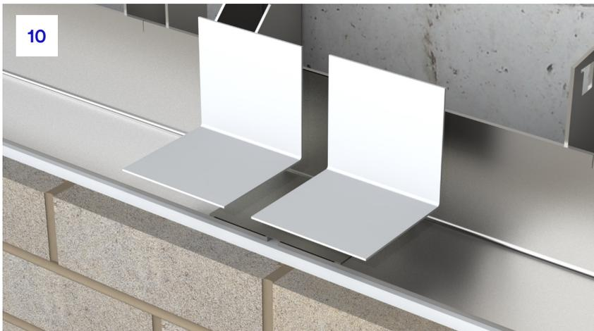
**10.** On top of each side of the jointing piece, a strip of single-sided ACS Butyl tape should be utilised. This should sit half onto the jointing piece and half onto the angle below.
