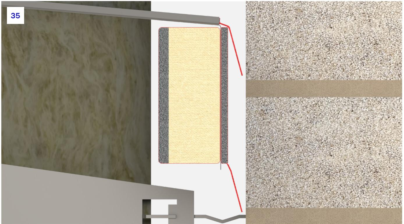
**35.** As brickwork continues up the façade, it is imperative that the barrier wings are left free within the cavity space. Under heat and fire, the wing expands into the brickwork to assist with intumescent expansion.
