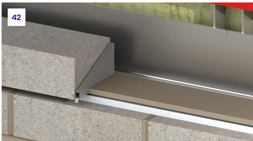
**42.** The system can be used with ACS stainless steel weep vents. These should be used on fresh mortar ensuring any moisture collected on the tray is ejected from the cavity. The lipped section of the weep vent should sit proud of the brickwork to ensure moisture is successfully ejected.
