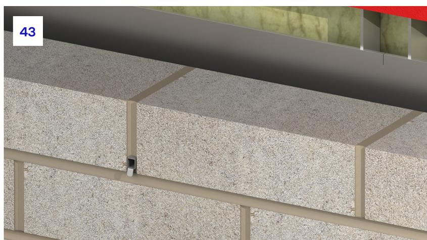
**43.** Mortar should be placed into the remainder of the vertical mortar joint to ensure the weep vent is sufficiently held in place.
