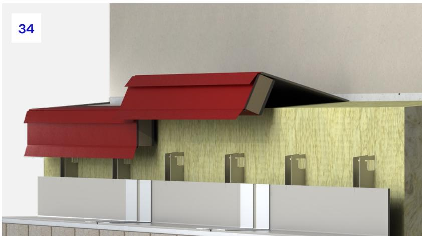
**34.** The tray can be fitted around the insulation ensuring a tight fit between all components.
