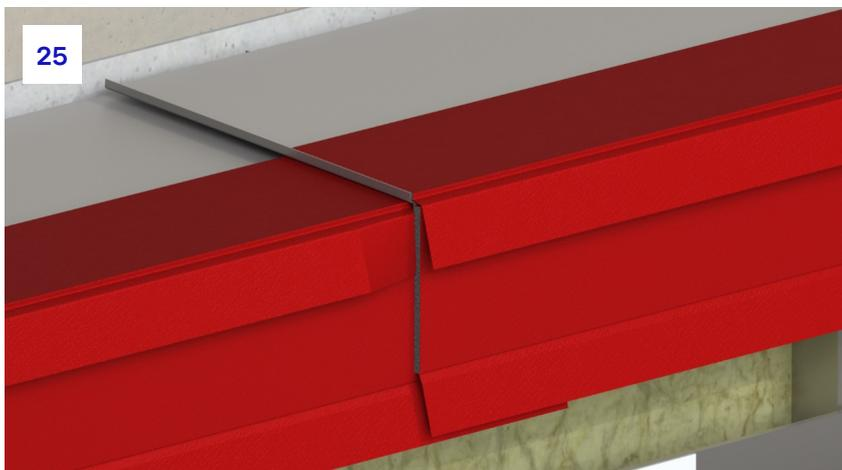
**25.** For both the top and front sections of the tray barrier, the second tray should sit on top of the lower barriers as shown in the image. This ensures continuity in the case of fire.
