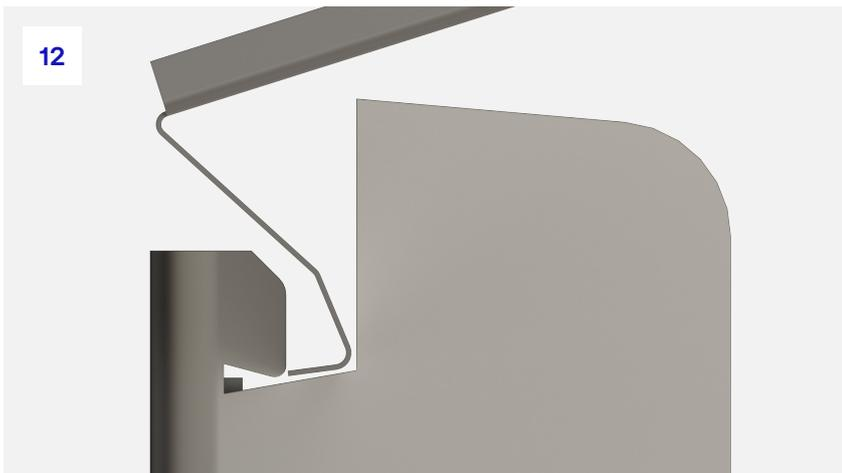
**12.** The bottom lip of the tray section should be pushed fully into the bracket notch to its rearmost face. The bracket notches are specially designed to match the profile of the tray.
