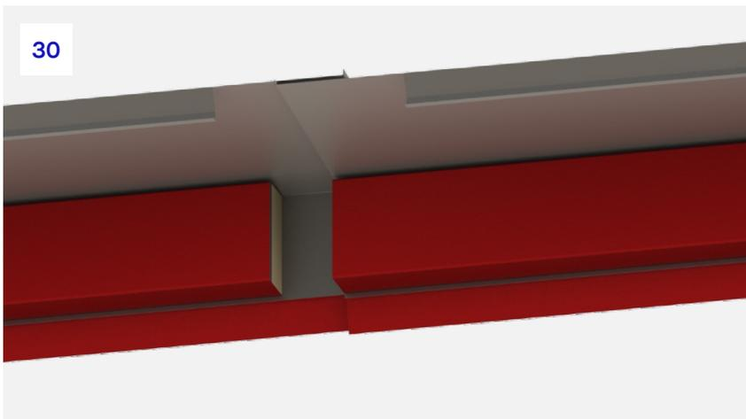
**30.** Once the rear barrier is cut the two barriers can be pushed together. For the rear section, the two barriers should be fully butted together to ensure they provide a continuous stop against heat and flame.
