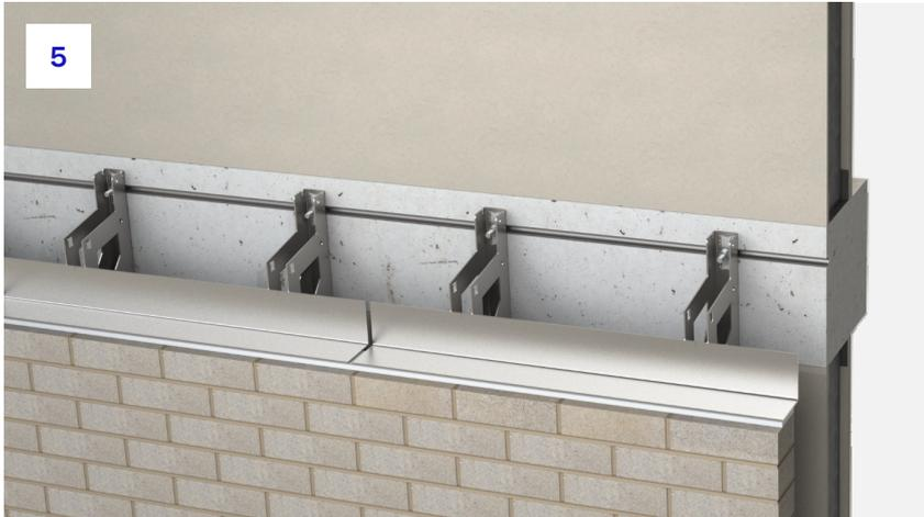
5. Continue to install further pieces of Intex™ brackets and angle, allowing for around a 10mm gap between units. Each angle should be levelled to the value shown upon the ACS drawings. A string line is commonly used to assist with installation. ACS drawings will show unit references which must be used to ensure the correct pieces are installed.
