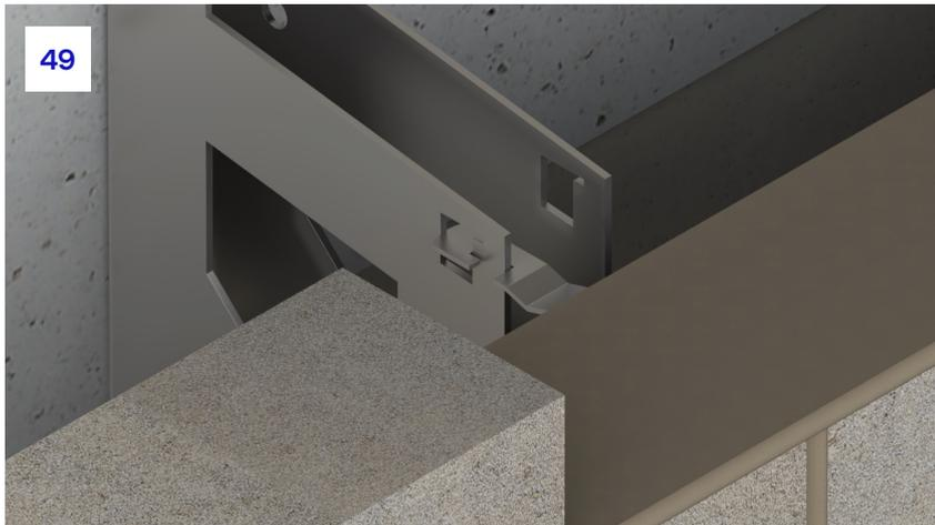
**49.** Further mortar should be placed on top of the tie to ensure it will have sufficient restraint against pull out. The next course of bricks can then be placed on the top of the mortar.
