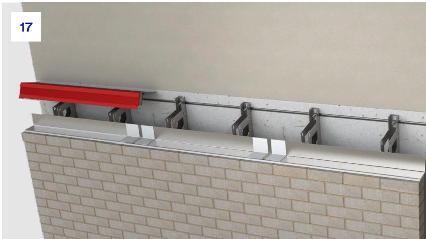
**17.** Once the insulation is in place, it is time to start the installation of the trays. For this section, the insulation has been removed from the images to help with clarity. The relevant first tray should be lined up with the adjoining vertical barrier or structure as per project-specific details. The rear section of the tray should be lined up with the slots in the tops of the brackets.
