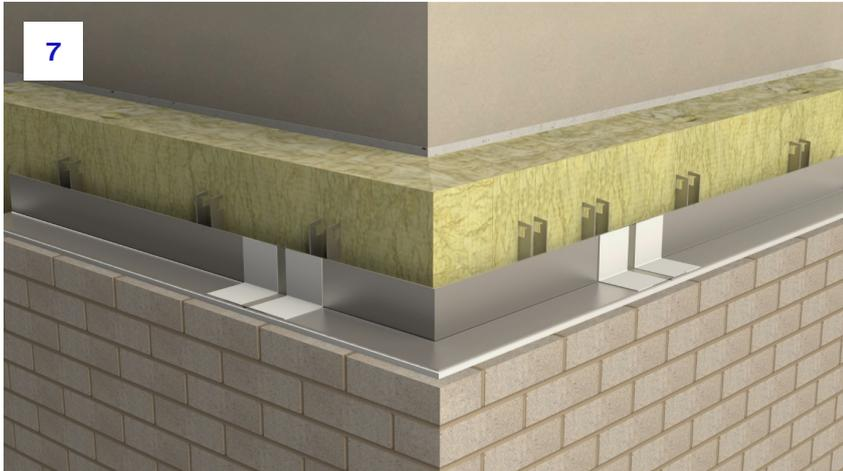
**7.** Thermal insulation should be tightly installed both between the bracket legs as well as between brackets ensuring it is tight up against all components to create a continuous face for the rear intumescent to expand against. For further details, please see the main section of the installation guide.
