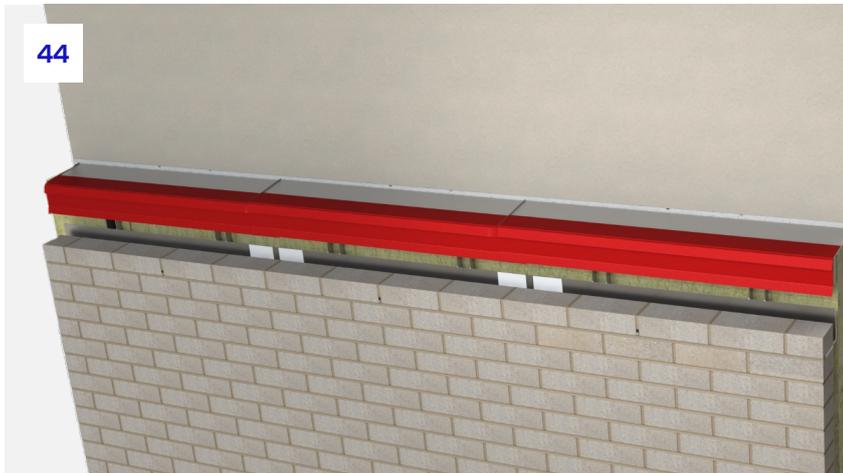
**44.** Centres for the weep vents should be specified by the project design team ensuring that water can be sufficiently ejected.
