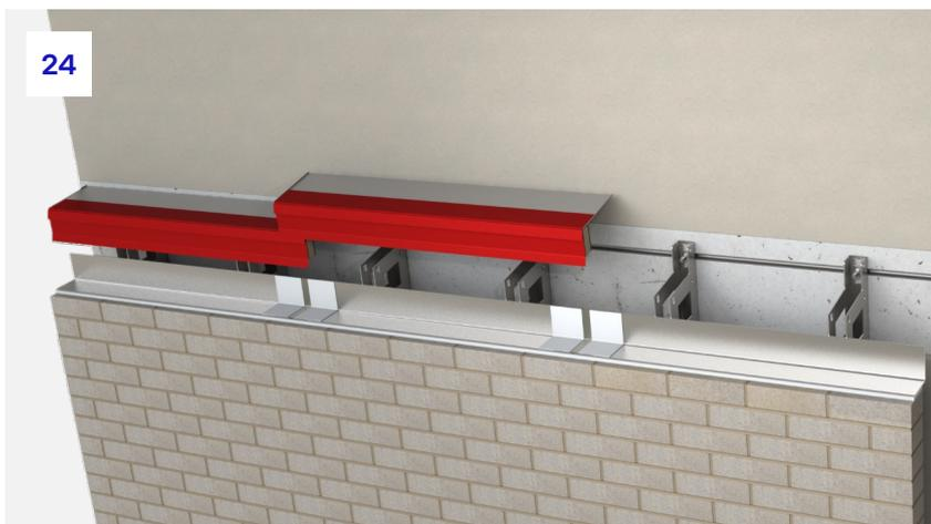
**24.** The next tray can then be placed on top with a minimum of 80mm overlap between components. Horizontal tolerance in the system is given by sliding the tray along the bracket slot detail.
