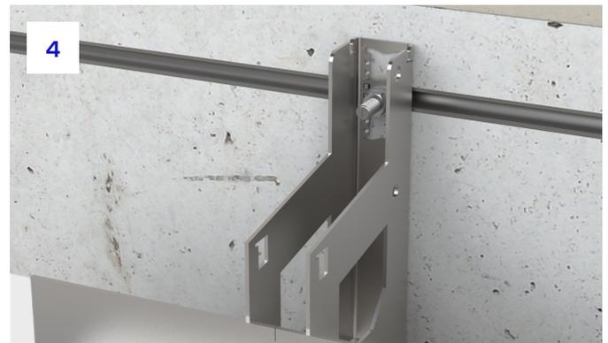
**3.** The ACS bracket contains the patented Alpha II adjustment methodology which can be used for required adjustment, offering  $\pm 25\text{mm}$  vertical tolerance. The washer can also be spun round  $180^\circ$  for fine adjustment between teeth. Please ensure that all minimum edge distances and fixing embedment depths are adhered to. For fixing specific information, please see relevant project approval drawings and fixing information.
