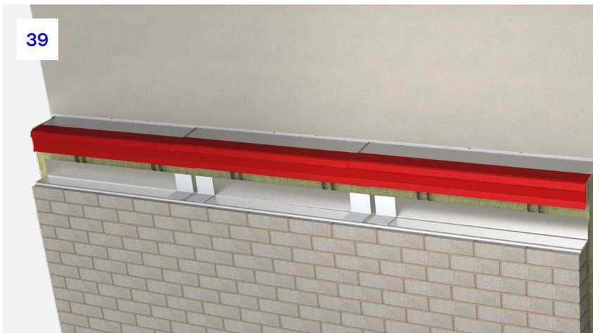
**39.** Once the second tray is in place, the same process can be followed for any remaining trays, ensuring the references match between the drawing, angle, and tray.
