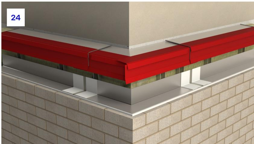
**24.** At this stage the corner wings will project past the corner into the brickwork area.
