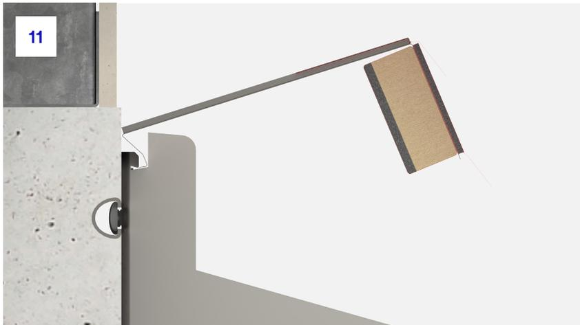
**11.** The tray should be tilted towards the vertical to allow the formed section to sit into the bracket notches.
