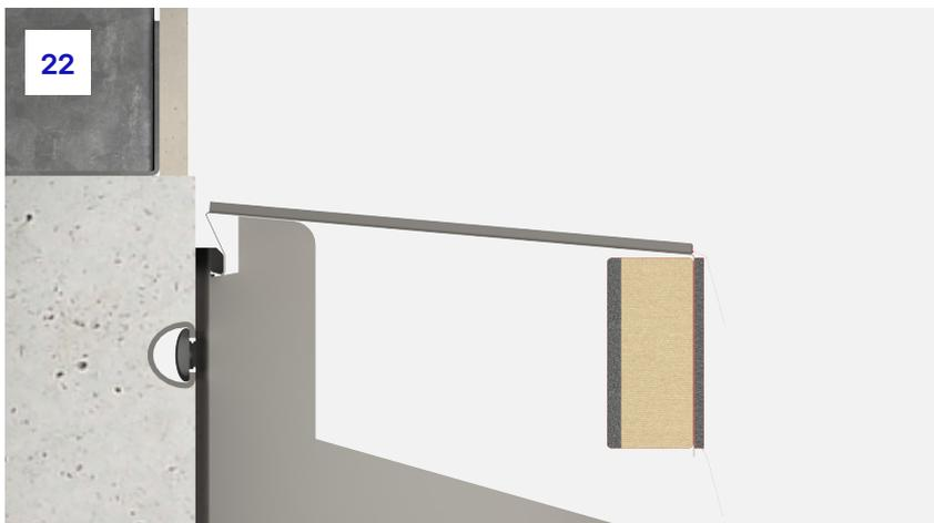
**22.** Once in place, the front face of the barrier should be parallel to the structure. This ensures any moisture which may fall onto the tray is directed towards the external face of the cavity.
