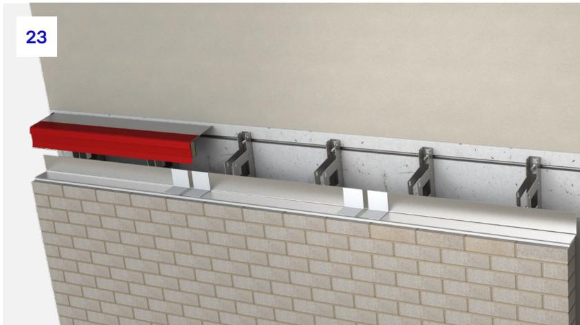
**23.** The tray must be inserted into all brackets along its length to ensure it is fully fixed in place.
