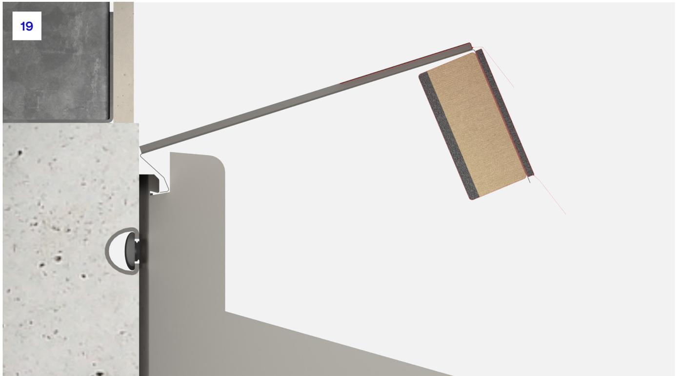
**19.** The tray should be tilted towards the vertical to allow the formed section to sit into the bracket notches.
