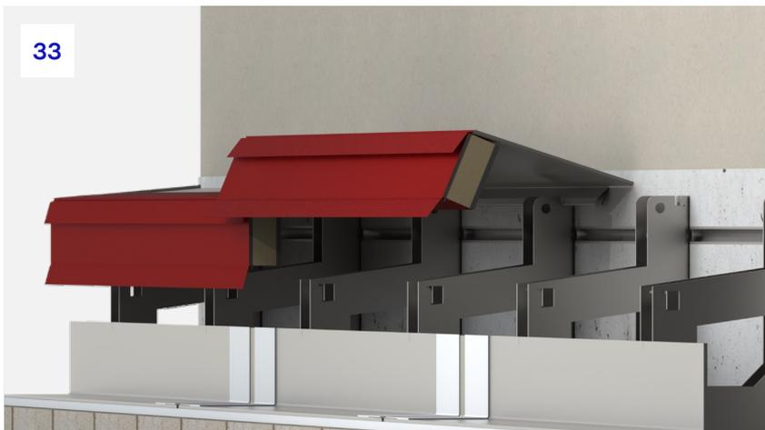
**33.** The bottom lip of the tray section should be pushed fully into the bracket notch to its rearmost face. The bracket notches are specially designed to match the profile of the tray.
