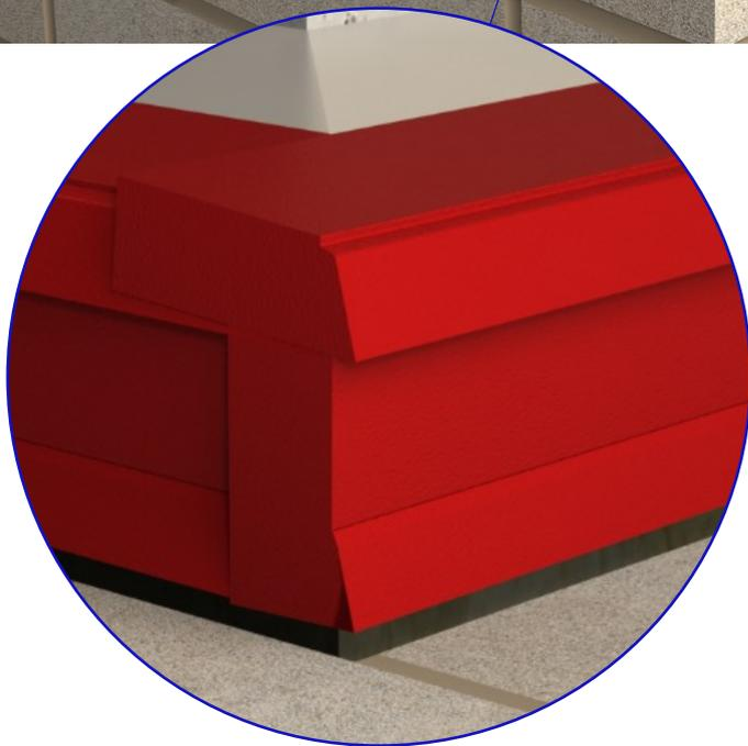
**32.** The same process should also be followed for the top intumescent strip, again ensuring that the wing is not built into the brickwork itself and is free to move under pressure in the case of a fire. More detail can be seen in the below image.
