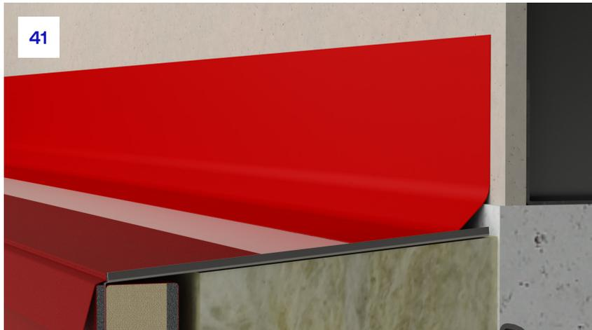
**41.** The membrane/tape should be fully sealed against both the internal structure as well as the Intex™ top tray as per manufacturer's guidelines.
