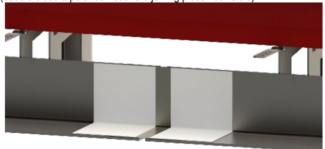
Diagram 4 - Fully sealed angle joint with joining piece and single-sided tape (double-sided tape underneath the joining piece not visible)
