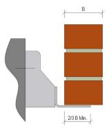
The maximum allowable thickness of shims should be no more than outside diameter of the fixing bolt or 16mm whichever is less. Larger cavity variation can be accommodated following the advice of the manufacturer.
