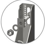
to be halved when rotated through  $180^{\circ}$  meaning the support level can be finely adjusted by +/-26.5mm. The design of the Alpha System provides clear inspection into the location and engagement of the washer in the bracket simplifying the final site installation checks.
