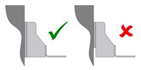
Shims should provide full bearing, ensuring the heel of the bracket is fully engaged with the structure to avoid excessive settlement and deflection under load.
